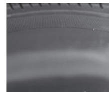
Under-Inflated Tire - An abrasion may run around the circumference of the tire and wrinkles may be observed in the inner liner.
